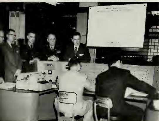
5. Tape is then processed through the Computer which automatically updates the files and singles out items for the attention of the supply manager.
